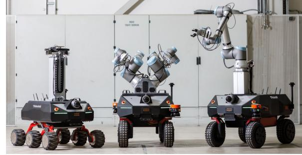
Three robots are available to experimentally validate the developed algorithms (see figure). These are operated on the software side using the Robot Operating System, or ROS for short. Various tasks, such as sequential logic systems, controls, monitoring, etc., have to be implemented in ROS (Python, C++) .
